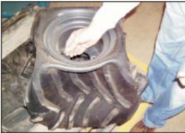
Figure 11-8. Replacing the Valve.
