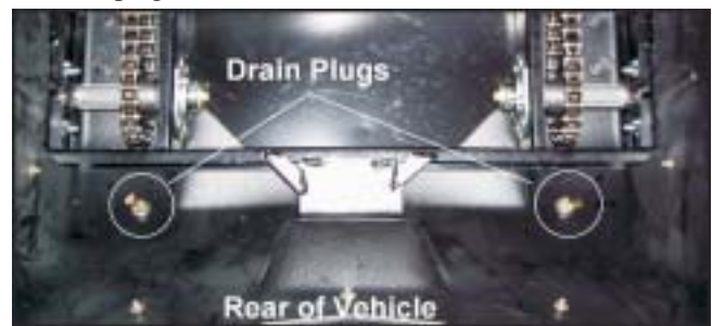
Figure 5-1. Location of rear drain plugs
