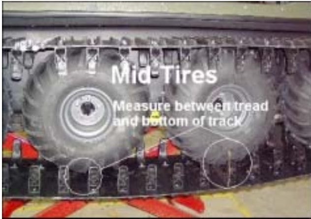
Figure 11-10. Measuring the gap of the mid tires.
