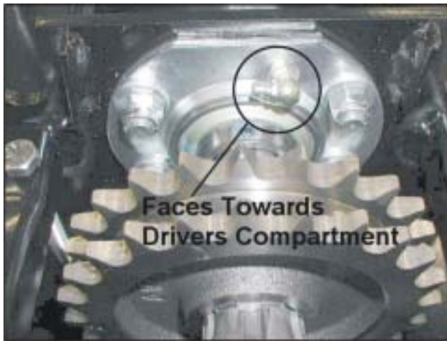
Figure 6-11. Idler shaft bearing grease nipples.
